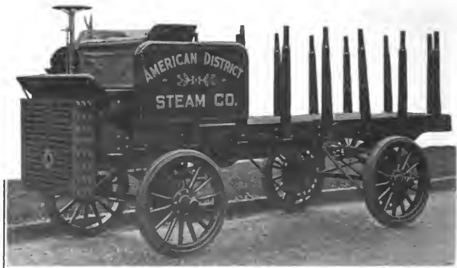
— TWO-TON "AMERICAN" STAKE TRUCK WITH FOUR-CYLINDER VERTICAL ENGINE.
